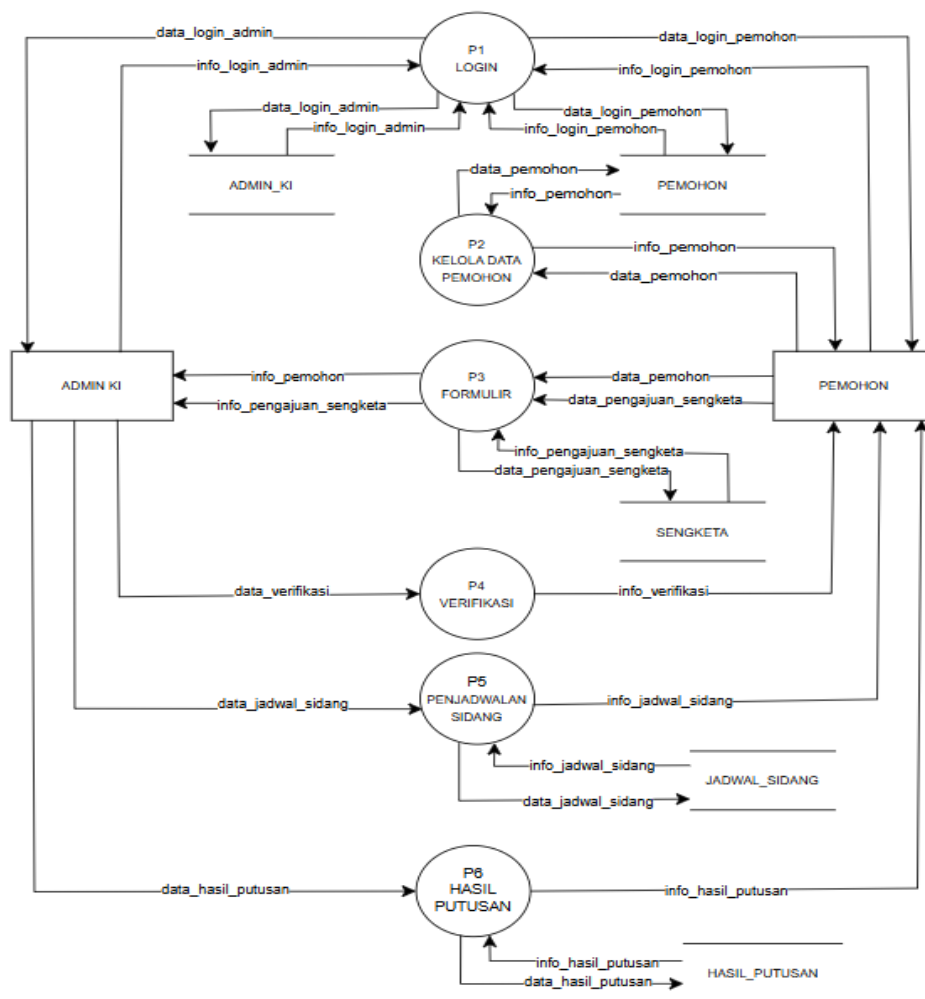
Gambar 4.2 Data Flow Diagram (DFD) level 0
